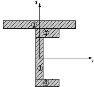
$$I_y = \frac{20 \times 120^3}{12} + 2 \times \frac{120 \times 20^3}{12} + \frac{240 \times 20^3}{12} + 2400 \times 36^2 + 2400 \times 34^2 + 2400 \times 106^2 + 4800 \times 54^2 = 50.05 \times 10^6 \text{ mm}^4$$
