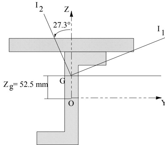
$$I_z = \frac{30 \times 360^3}{12} + 2349 \times 10^4 = 140.1 \times 10^6 \text{ mm}^4$$
